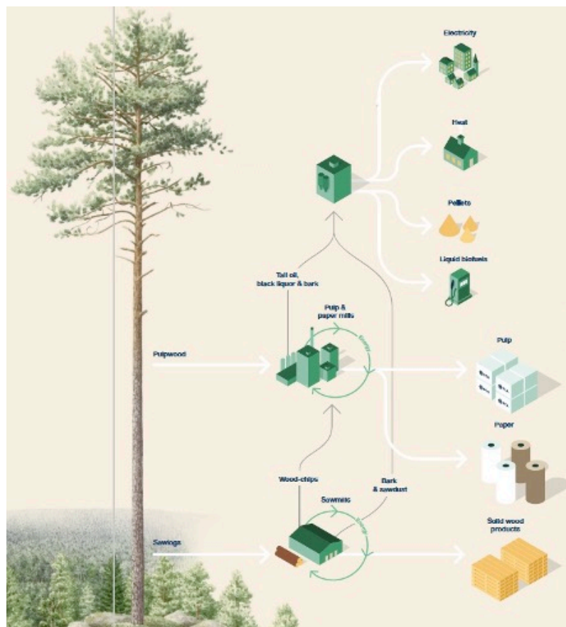
Figure 4. Illustration of how all stem biomass is used for a variety of products, in this study aggregated into (a) solid wood products, (b) fibre products, and (c) bioenergy. (Based on SCA Annual Report 2019, p.9)
